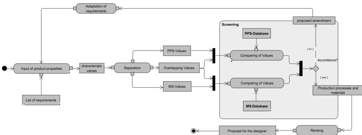
Figure 6. Activity diagram production process and material selection
