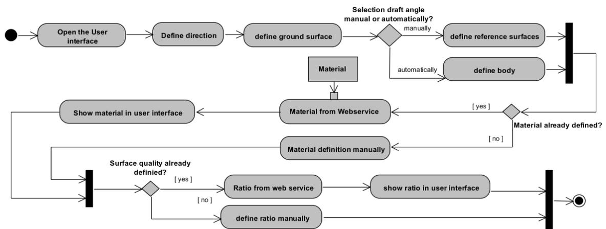
Figure 7. Activity diagram feature draft angle
