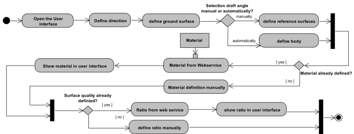
Figure 7. Activity diagram feature draft angle
