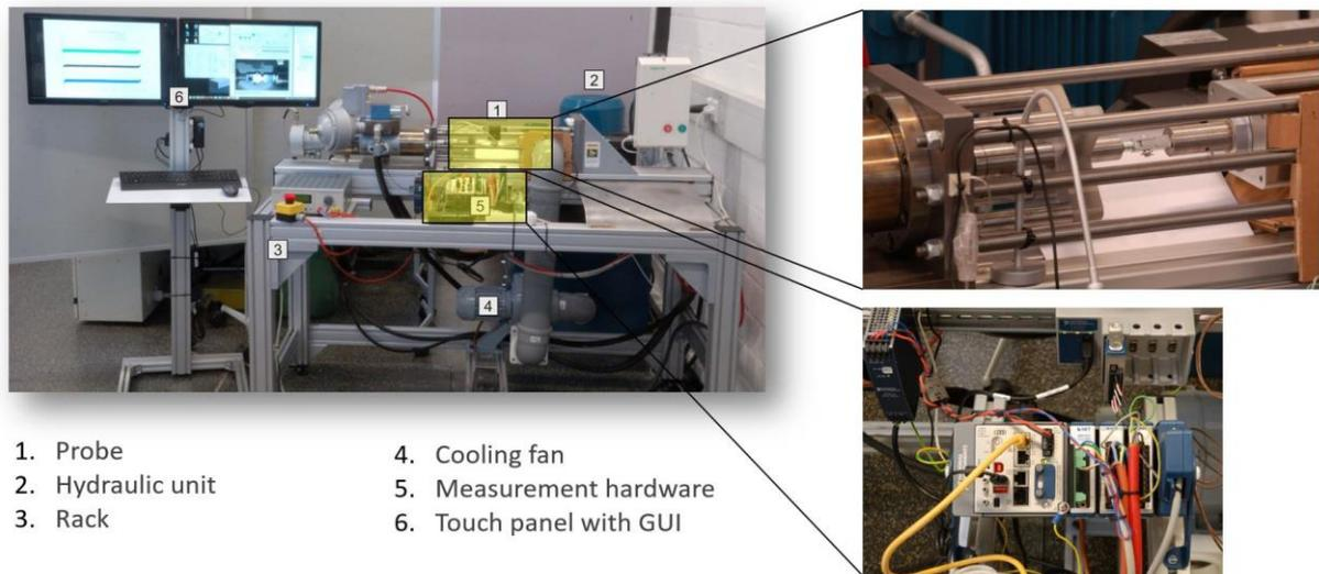
Figure 10. Overview of the experimental test rig
