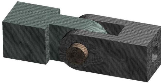
Figure 6. Mesh of the assembly
