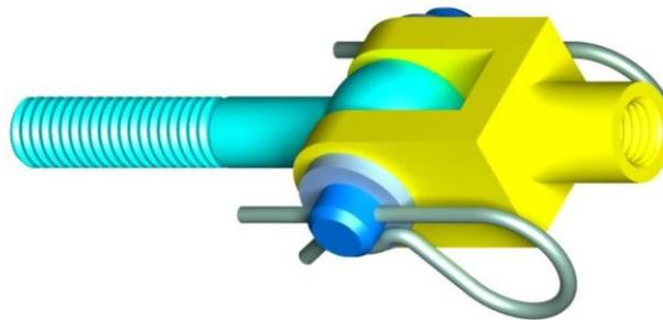
Figure 2. Machine Element: Clevis joint with bolt linkage
