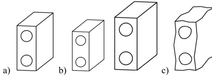
Figure 1. a) The nominal Geometry, b) The nominal geometry with maximum and minimum dimensional tolerances c) The non-ideal representation of a geometry, Source (ISO 17450-1, 2012)
