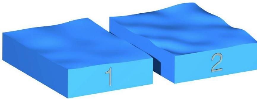
Figure 5. Variants for the creation of non-ideal surfaces (amplified)
