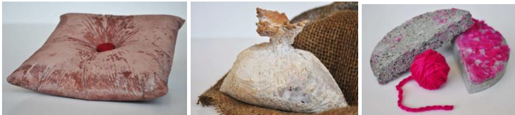
Figure 2. Experiments from product design student Anne Gerd Eira: How to make concrete look more like a soft, warm and lightweight material.
