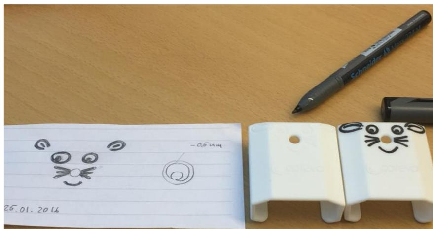
**Figure 10: The end result of the development experiment showing the PAD-draft, the 3D printing outcome and result after that the marker pen had been used to fill in the “ditches”**
