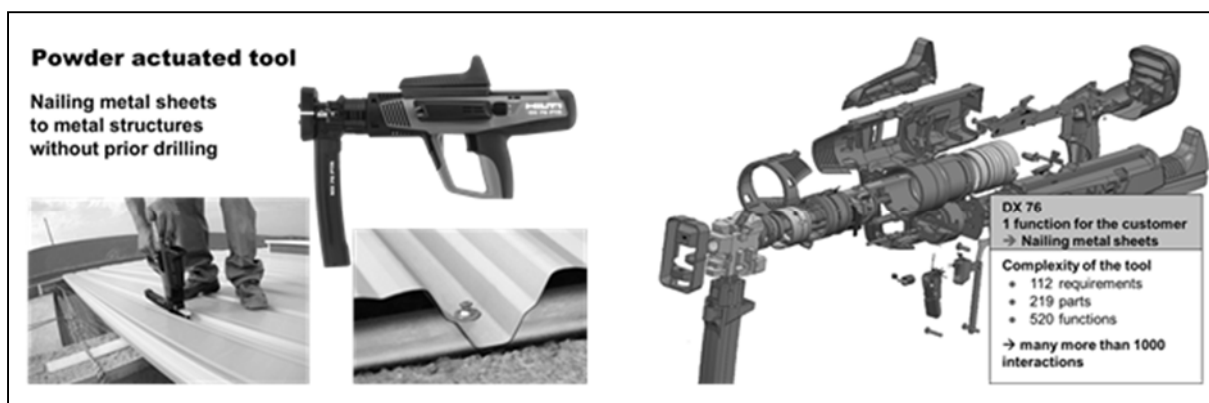
Figure 3. Power-tool with over 500 functions realized in the embodiment [Matthiesen 2011]
