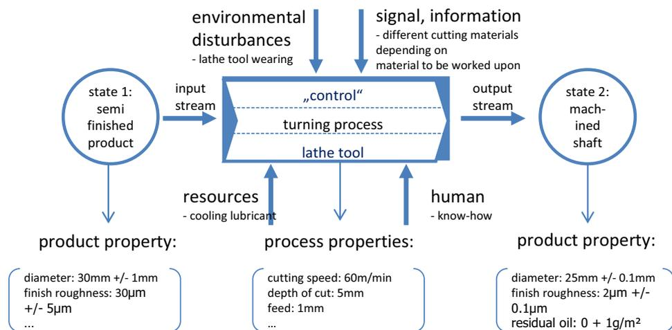
Figure 2. Process model at the example of a turning process
