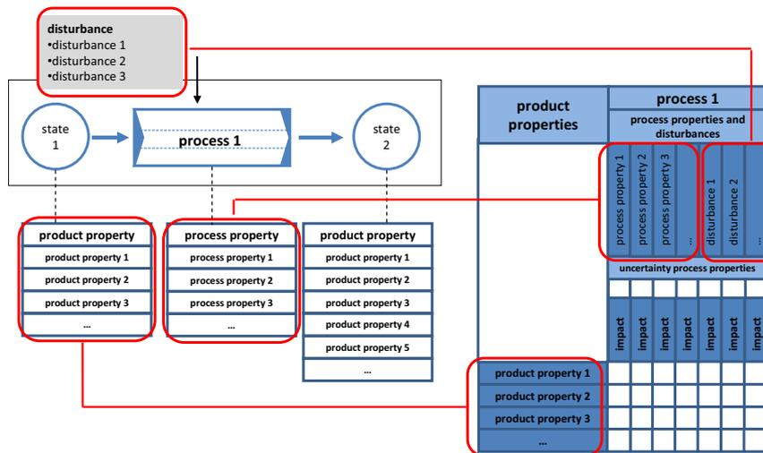
Figure 4. Step 1 – Classification of process properties and disturbances
