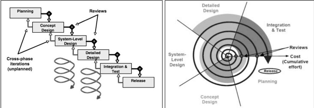
Figure 1: Waterfall (left) and spiral model (right) [6]
