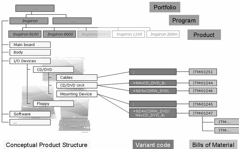
**Figure 3. The connection of the conceptual product structure to the BOM [Zagel, 2006]**
