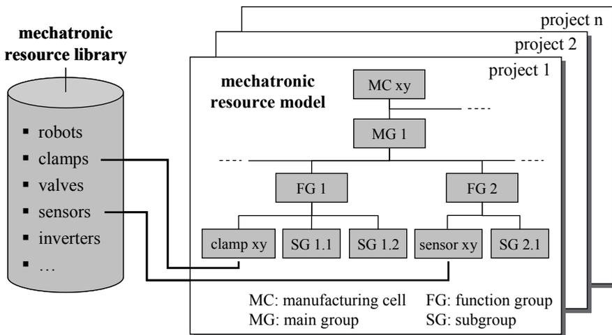
**Figure 3. Data structure of a cell-specific mechatronic resource model**
