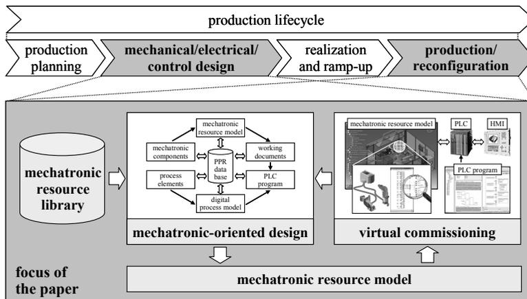
Figure 1. Focus and aspects of the mechatronic-oriented design methodology
