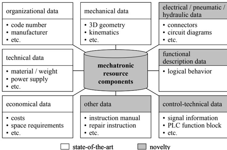
**Figure 2. Contents of a mechatronic resource component**
