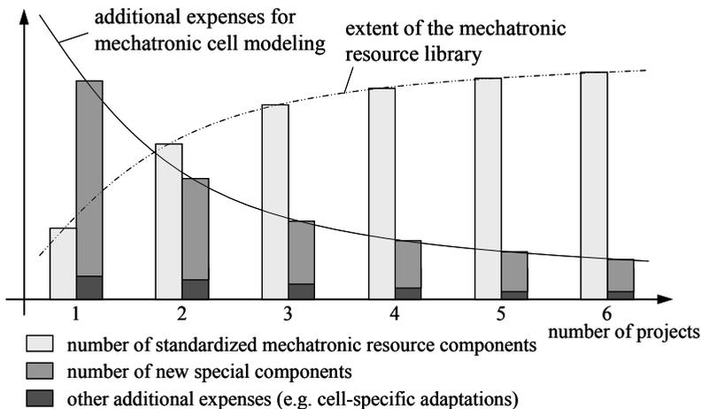
**Figure 5. Reducing additional expenses for mechatronic cell modeling**
