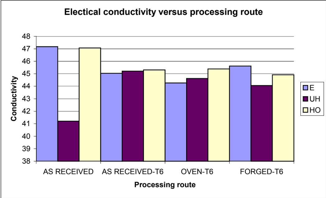
Figure 8. Electrical conductivity of test specimens versus processing route. Legend: E – extruded, UH – unhomogenised, H – homogenised.
