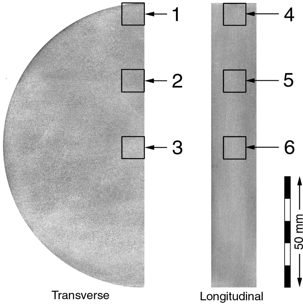
Figure 6. Unhomogenised billet section, caustic soda etch (50°C for 80 seconds)
