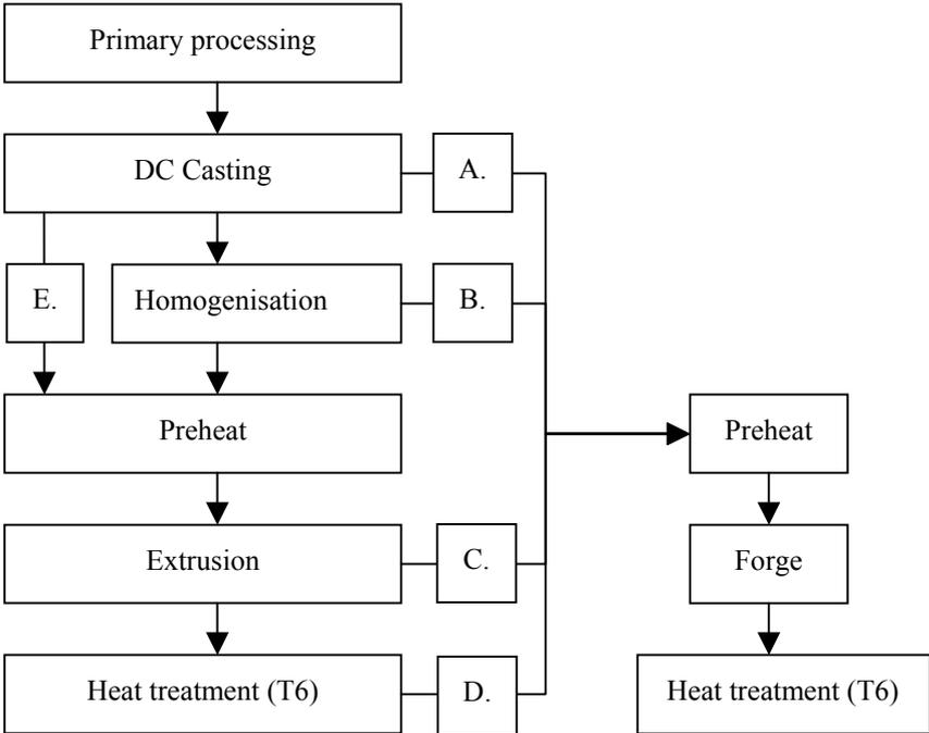
Figure 1. The feasible processing paths for the proposed material as identified by material suppliers, tier-one forging manufacturers and reference to the available literature. Processing path D is currently applied by the forging supplier. Processing path E. was identified as feasible, but was not considered cost effective by the material supplier. Processing paths A and B have been identified as opportunities to reduce the contribution of the processing path to the component cost.
