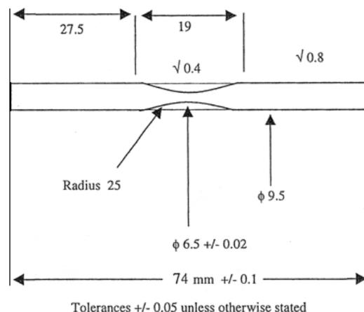
Figure 10. Fatigue strength specimen geometry
