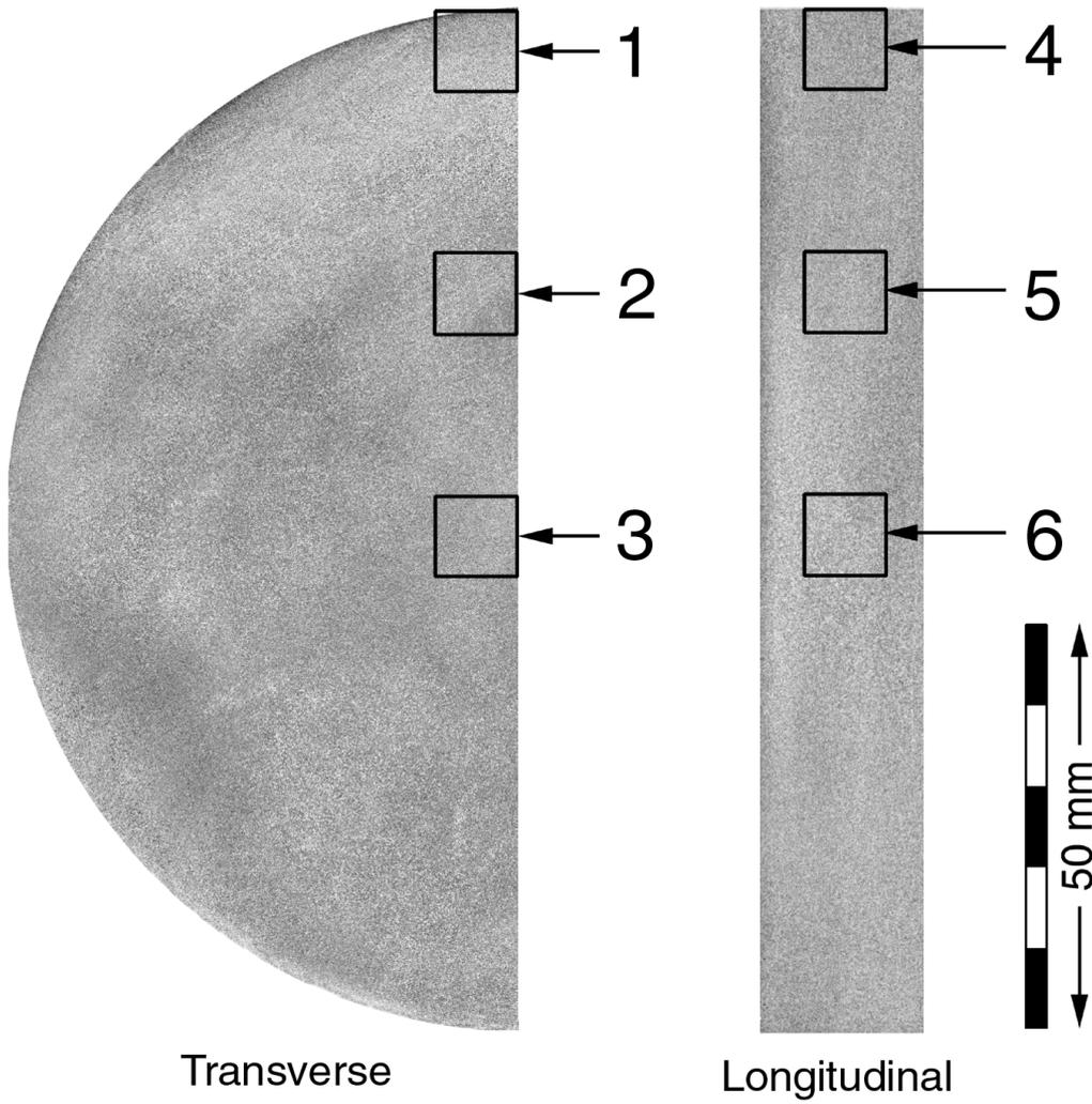
Figure 4. Homogenised billet section, caustic soda etch (50°C for 80 seconds)
