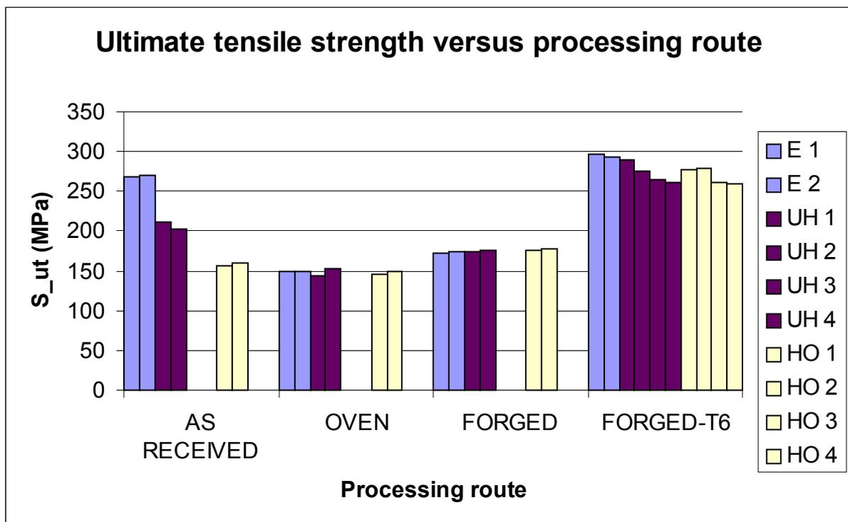
Figure 9. Tensile strength of test specimens versus processing route.
