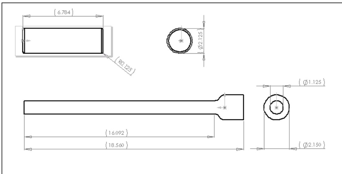
Figure 2. Initial billet geometry and subsequent extrusion. Unit of measurement: inches.
