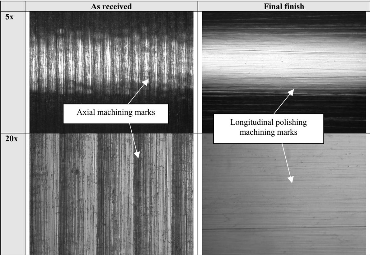
Figure 11. As received and final finish of fatigue specimens
