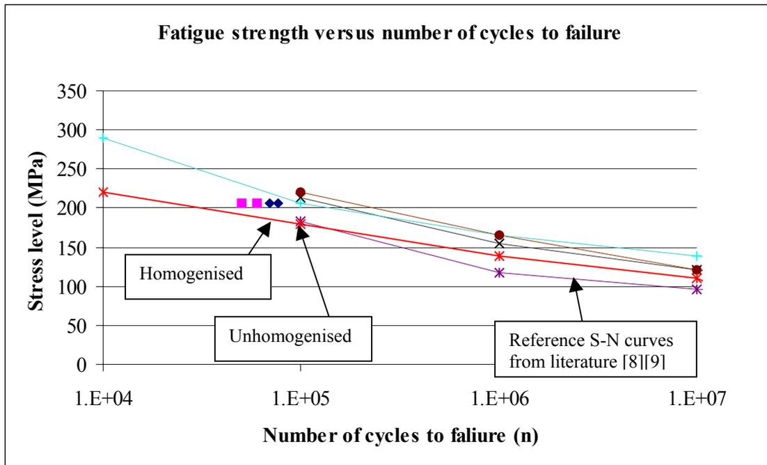
Figure 12. Fatigue strength of the proposed processing routes and samples available from the literature.
