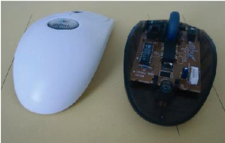
Figure 1 Optical mouse and its components
